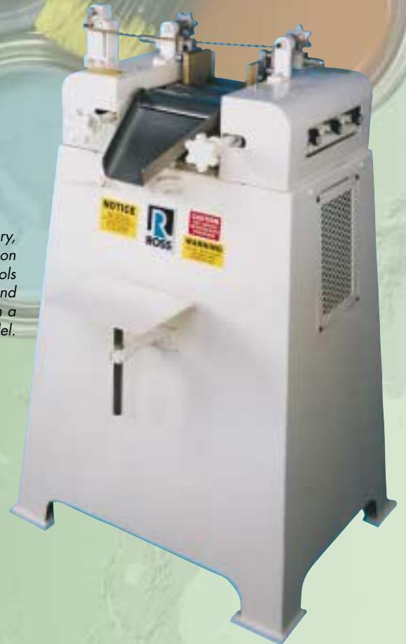
**The Model 52TC-9x24"** – is the workhorse designed for higher volume production operations. The hardened, precision ground rolls are cored for uniform cooling. This mill is built with longevity in mind and can be supplied with many optional features such as single point hydraulic roll setting controls, rotary pressure joints for forced heating or cooling of the rolls. Complete electrical control systems are also available.
