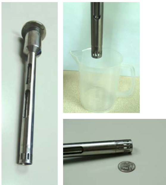
One rotor and one slotted stator
