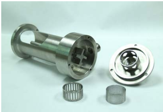
Inline High Shear Mixer (HSM) One rotor and three stators*
